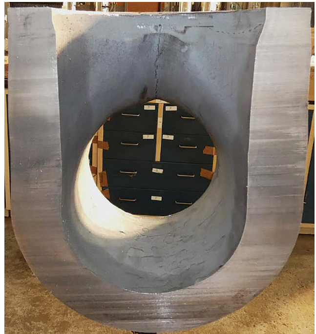
Fig. 2 — A through-wall crack in the crotch position on one side and a partial crack on the opposite side of the tee, originating from the inside diameter. There were cracks at the toe of both run and branch girth welds originating from the outside diameter. (Photo credit: Combustion Engineering Solutions [CES-ATC].)
