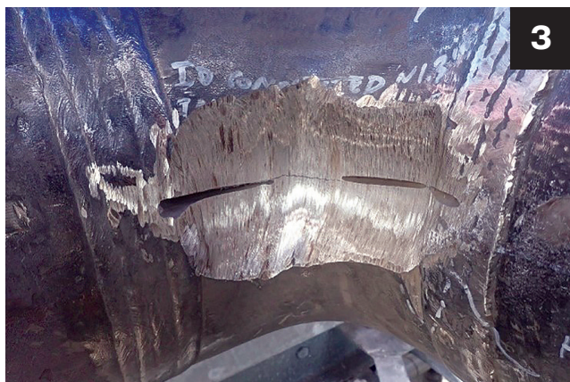
Fig. 4 — This crack was found using phased array ultrasonic testing (PAUT). Once plotted, a repair plan was developed and the welders excavated the crack to just before breaking the system open. Preheat was applied and the weld repair began until flush with the contour of the tee. (Photo credit: Combustion Engineering Solutions [CES-ATC].)
