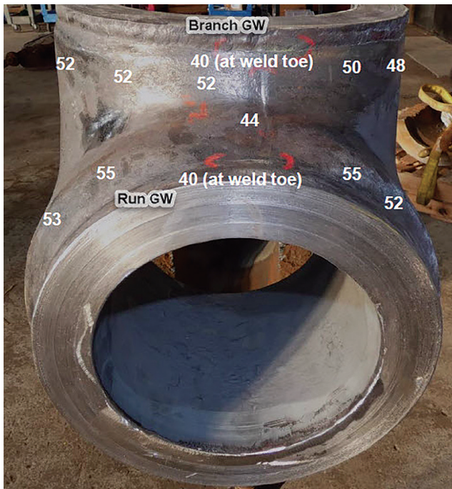
Fig. 1 — The through-wall thickness at the weld toes was 40 mm and below the minimum values. (Photo credit: Combustion Engineering Solutions [CES-ATC].)
