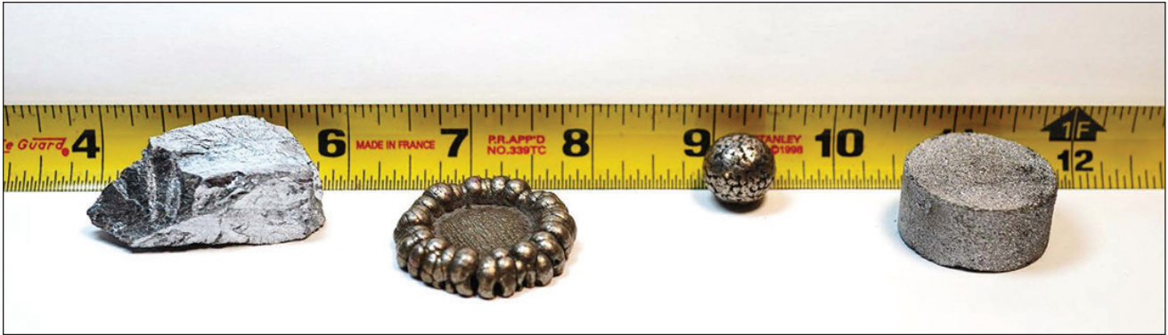
The feedstock for VIM: (from left) chromium, cobalt, nickel, and molybdenum.
