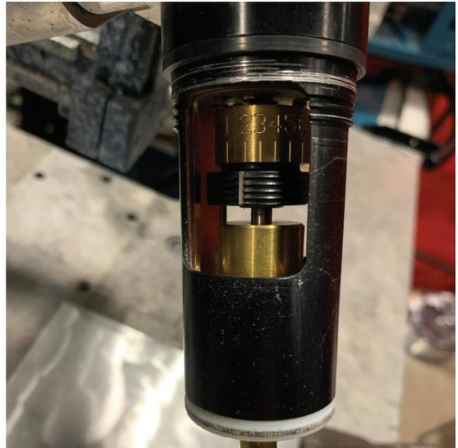
*Fig. 2 — Spin diameter adjustment on the SpinArc gun.*
