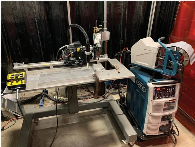
*Fig. 1 — REP-GMAW equipment setup. Bug-O tractor with OTC Welbee 500 GMAW power source and wire feeder.*
