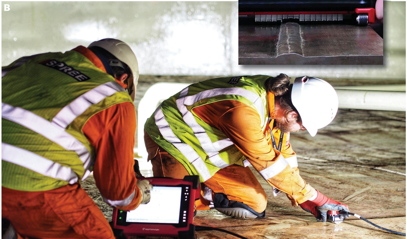
Fig. 4A – Newer ACFM probes feature increased crack detection and sizing performance using micro sensors instead of mini sensors; B – ACFM instruments enable rapid scanning with the handheld probe, reliable crack detection and characterization, reduced cleaning requirements, and a digital data record for backup, offline, and audit purposes.
