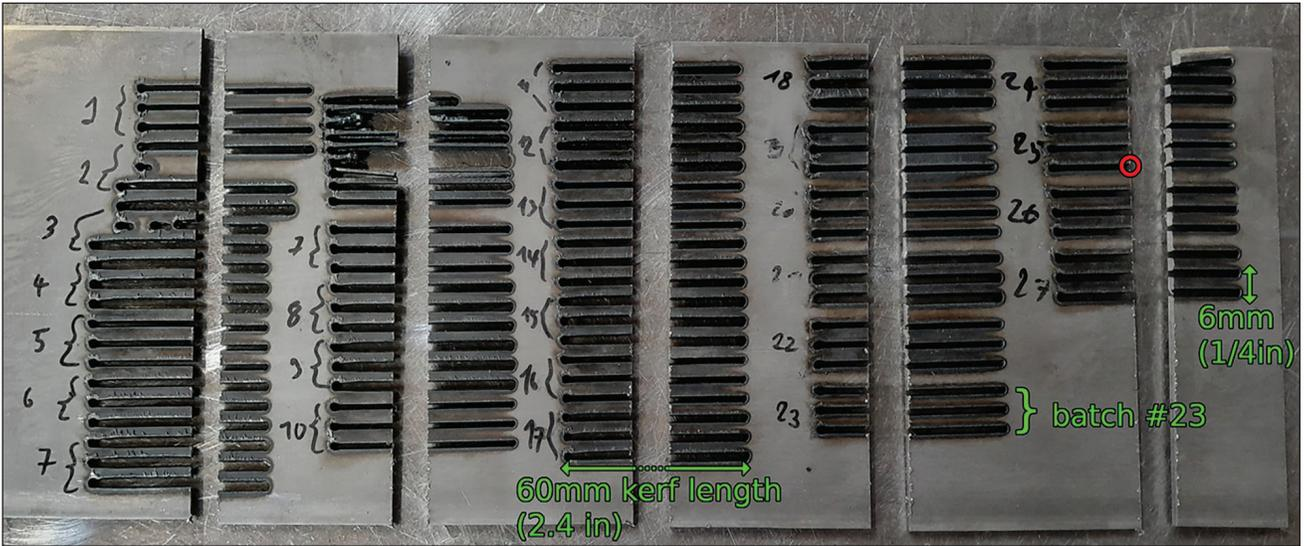
Fig. 3 – Samples after they were saw-cut: the numbers are those of the sets of parameters; the red circle is where Figure 4 was shot.
