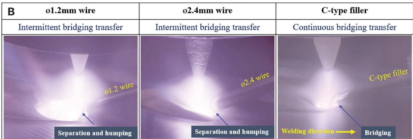
Fig. 13 – A – Comparison of metal transfer modes between the welding wires and C-type filler metal at a DR of 5 kg/h ( $I = 500$  A,  $U = 60$  cm/min); B – in-situ welding camera images of the filler metal’s melting edge and molten bridge for the welding wires and C-type filler metal at a DR of 5 kg/h ( $I = 500$  A,  $U = 60$  cm/min).
