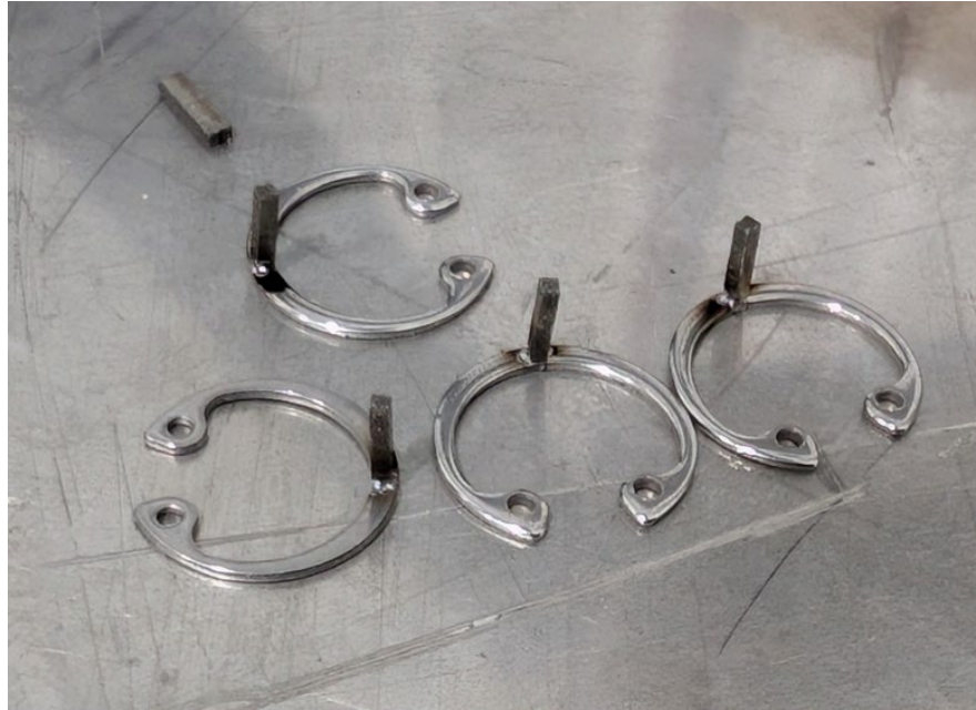
Figure 23: Photograph showing stainless steel internal diameter retaining rings (snap rings) with 'post' feature produced using HLBW with individual laser pulses of 12 J [courtesy of Apollo Machine, Canada].
