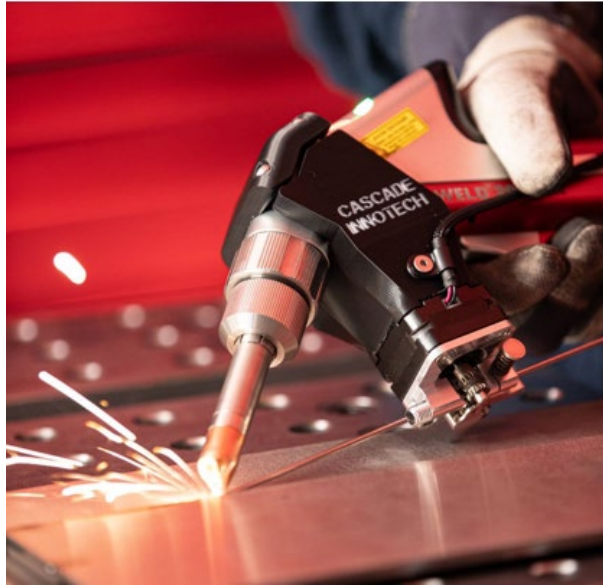
Figure 5: Filler metal feeding system for use with TIG rods (courtesy of www.LaserTug.com , USA).
