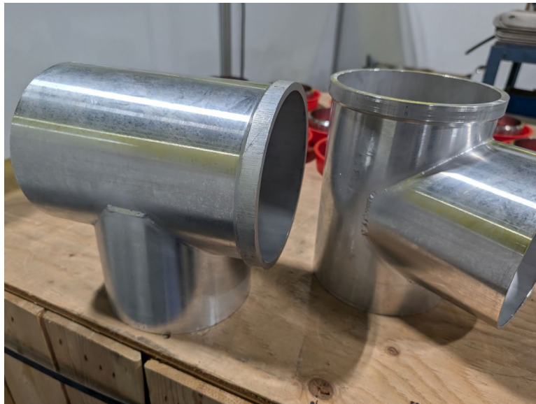
Figure 29: Thin walled fabrication using 6061-T6 aluminum welded using HLBW with ER5356 filler wire [courtesy of Apollo Machine, Canada].
