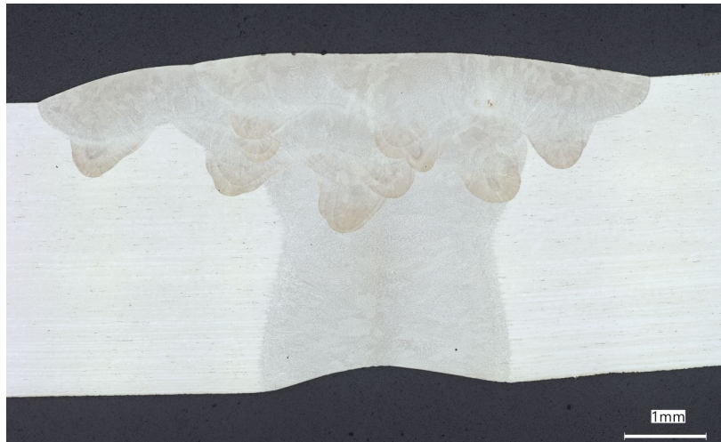
Figure 28: Single side welding of IN 625 tube with matching filler wire produced using HLBW [courtesy of Apollo Machine, Canada].
