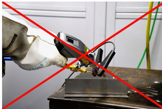
Figure 11: Photo showing contact tip to work bypass [courtesy of ifw Jena, Germany].
