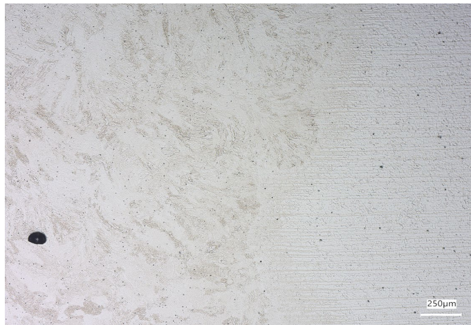
Figure 24: Light micrograph showing the approximately 0.2 mm wide heat affected zone (HAZ) between carbon steel weld metal (left) and unaffected base metal (right) produced using HLBW [courtesy of Apollo Machine, Canada].
