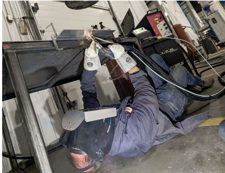
Figure 18: Overhead welding with HLBW [courtesy of Apollo Machine, Canada].
