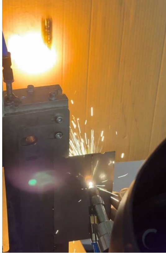
Figure 10: Beam energy passing the sheet in blind seam welding and ignites cardboard on the wall [courtesy of ifw Jena, Germany].
