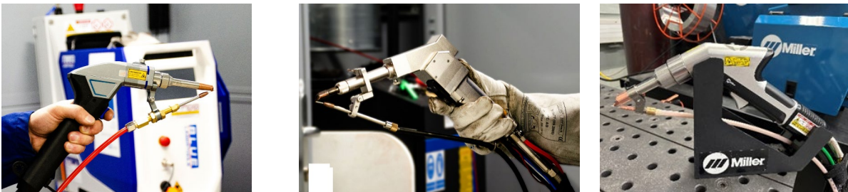
Figure 1. Laser heads with single-axis (left) and two-axis (middle) beam oscillation and with active plasma monitoring (right) [courtesy of ifw Jena, Germany, and Miller Electric Mfg LLC, USA].
