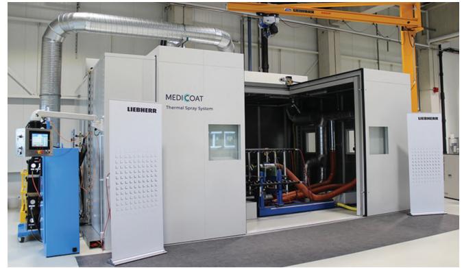
The latest HVOF technology is applied in Liebherr-Aerospace Lindenberg's new building for surface treatment. (Photo copyright of Liebherr.)
