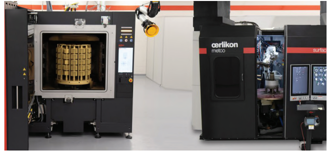
Inside Oerlikon's new Advanced Coating Technology Center, the INNOVENTA kila and Surface One™ coating machines offer PVD and thermal spray capabilities, respectively.
