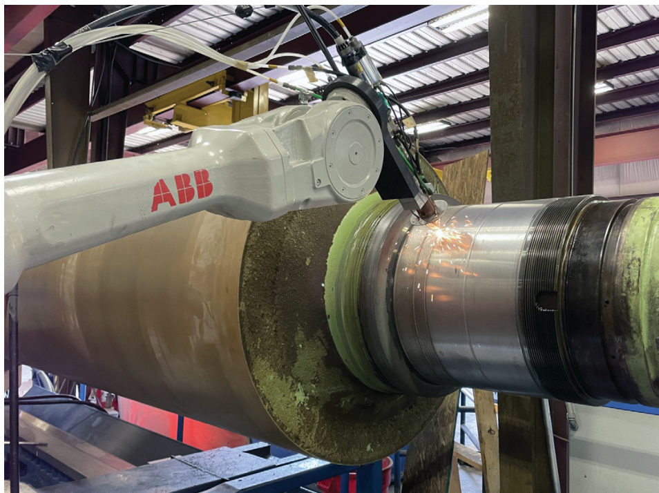
Laser cladding of a massive roll journal at a customer's facility in New Hampshire.
