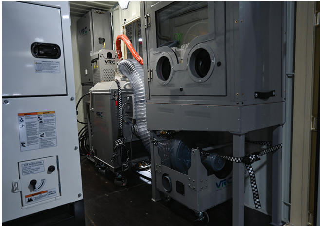
A portable cold spray enclosure unit and dust collector sit inside a Mobile Cold Spray System trailer at Ellsworth Air Force Base, S.Dak. (U.S. Air Force photo by Airman 1st Class Dylan Maher)
