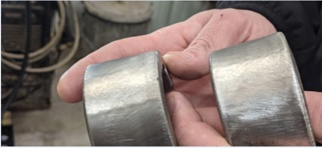
Chris Morr (left) and his son Devon prepare to bend parts during an AWS ATF audit. Sample test parts are also shown.
