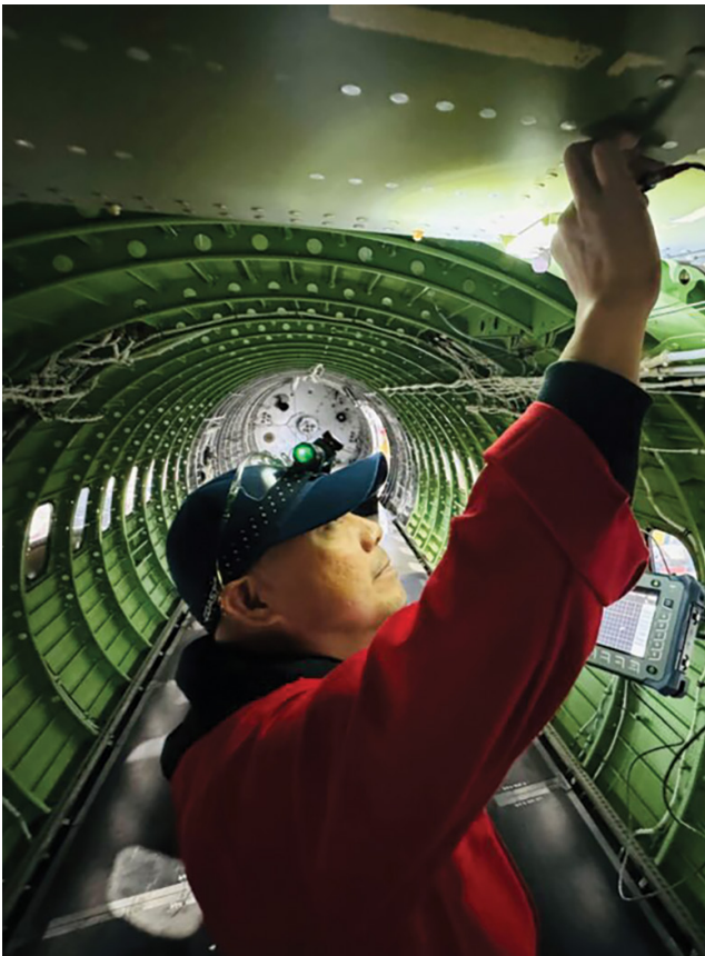
A Conair NDE technician performs eddy current testing on the interior of an aerial firefighting aircraft.
