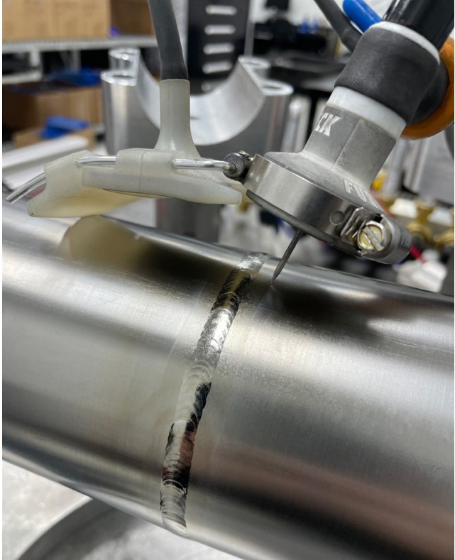
This view shows a butt joint for the start of a titanium airship hub.
