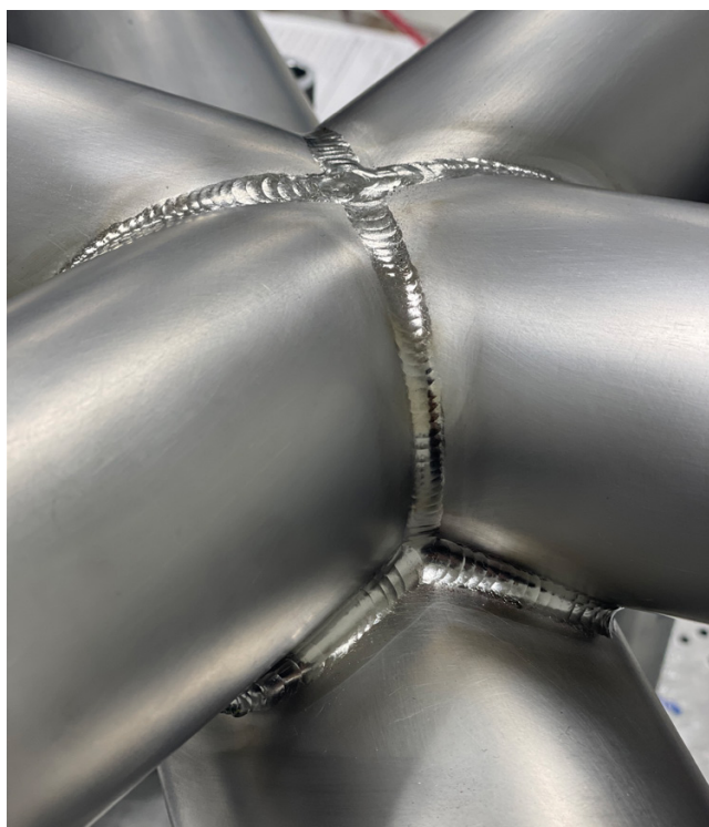
This image highlights a completed titanium airship hub.
