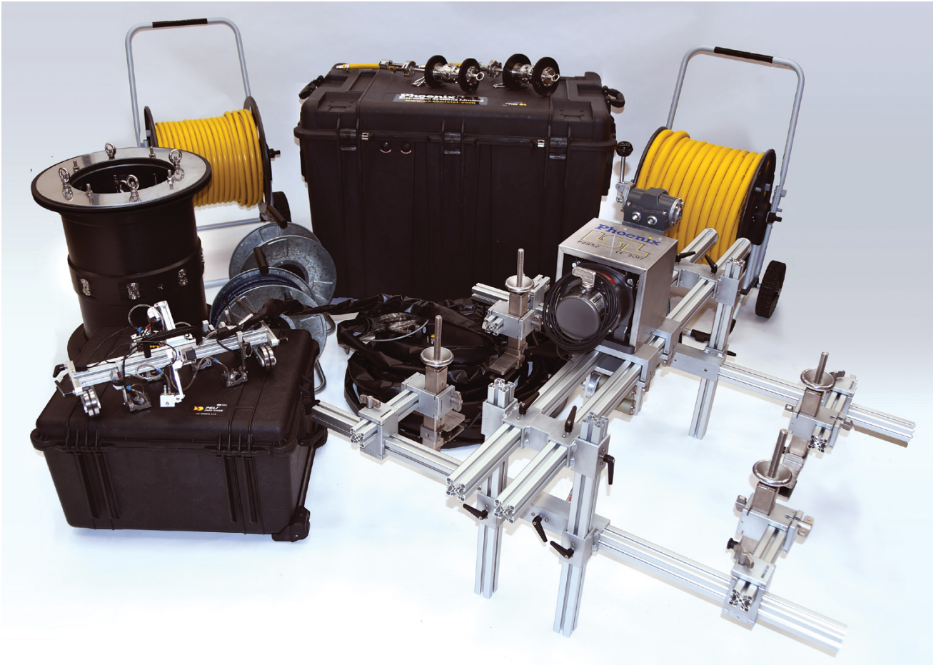
Fig. 1 — A Phoenix Inspection Systems Ltd. (Phoenix ISL) system for marine riser inspection.
