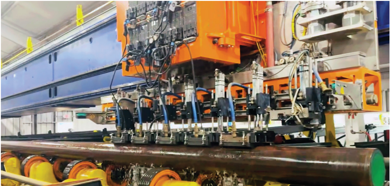
Texas Steel Conversion's new phased-array FLUT inspection line expands the company's NDE capabilities for steel tubular products.
