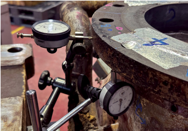
Fig. 3 — Distortion control setup during welding.
