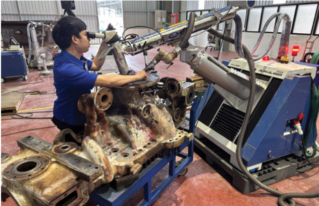
Fig. 3 — Distortion control setup during welding.
