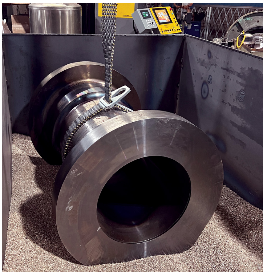
Fig. 6 — Immediately following hardfacing, the 700°–800°F valve body was placed in a bin and covered with vermiculite. It took a nominal four days for the valve body to cool down to room temperature.
