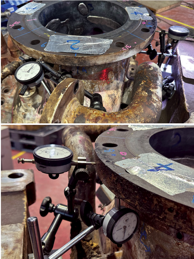
Fig. 3 — Distortion control setup during welding.
