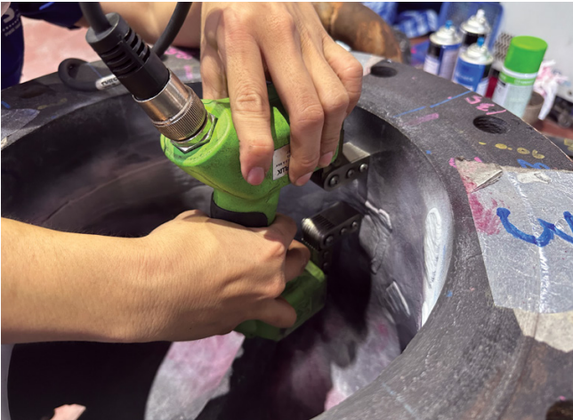
Fig. 5 — Magnetic particle testing.
