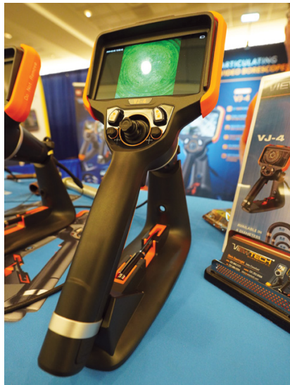
The VJ-4 from ViewTech Borescopes is its newest articulating video borescope, featuring a high-quality camera, intuitive navigation, on-screen annotation, and a reference measurement function.
