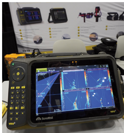
Sonatest showed its latest portable phased array detector, the Veo3 , suitable for weld inspection, corrosion mapping, and composite testing. The detector features real-time, multiscan/multitechnique capabilities, including TFM, PAUT, and TOFD.
