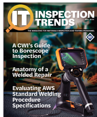
COVER PHOTO: A handheld articulating video borescope used for remote visual inspection. (Credit: ViewTech Borescopes.)
