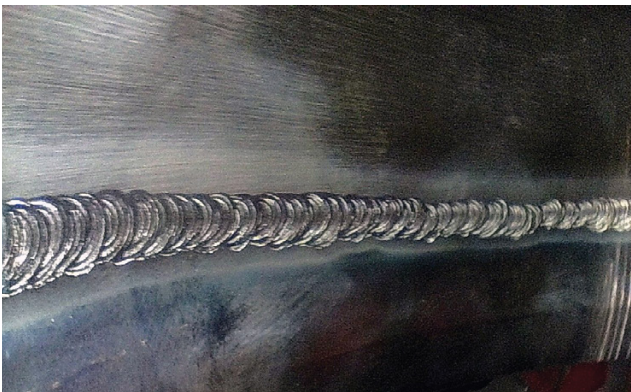
Fig. 2 – A borescope image showing adjusted lighting, avoiding blooming.
