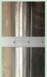
Fig. 1 — An American Society of Mechanical Engineers (ASME) Section III welding. Left — Orbital gas tungsten arc welding (GTAW), 6G interpass weld beads. Pipe material: P-No. 1. Center and right — Test weld joints in evaluating new weld filler metals using mechanized GTAW. Plate material: P-No. 43.
