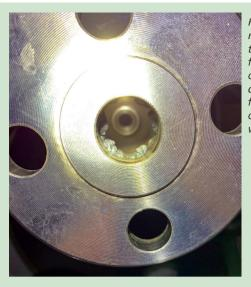
Fig. 4 — Pipe melt-through that resulted from the outside diameter fillet welding of the socket weld.
