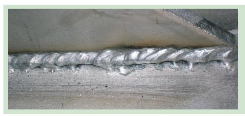
Fig. 3 — A poorly executed aluminum weld on a structural weldment.
