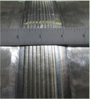
Fig. 5 — Top — Orbital GTAW narrow groove welding for a nuclear project. Pipe material: P-No. 1. Bottom — Orbital GTAW, 5G cap passes for a seismic oilfield project. Pipe material: P-No. 5A.
