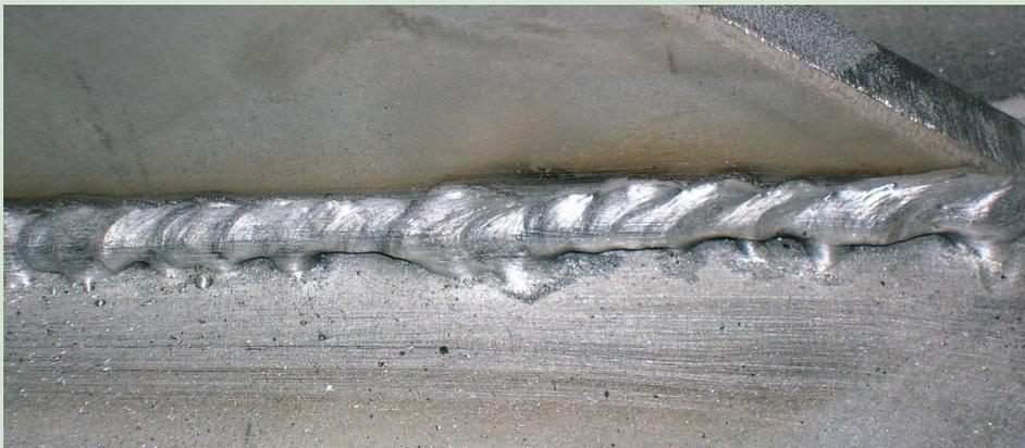
Fig. 3 — A poorly executed aluminum weld on a structural weldment.
