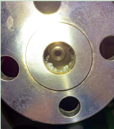
*Fig. 4 — Pipe melt-through that resulted from the outside diameter fillet welding of the socket weld.*
