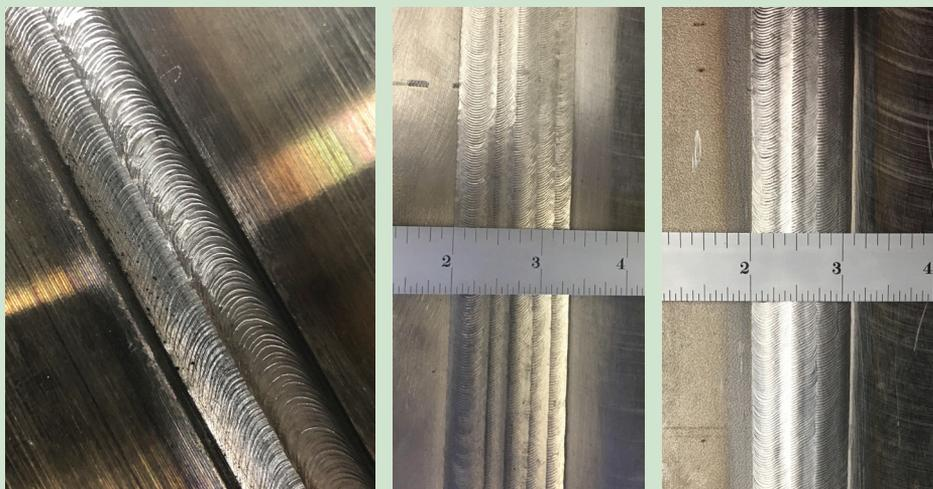
*Fig. 1 — An American Society of Mechanical Engineers (ASME) Section III welding. Left — Orbital gas tungsten arc welding (GTAW), 6G interpass weld beads. Pipe material: P-No. 1. Center and right — Test weld joints in evaluating new weld filler metals using mechanized GTAW. Plate material: P-No. 43.*
