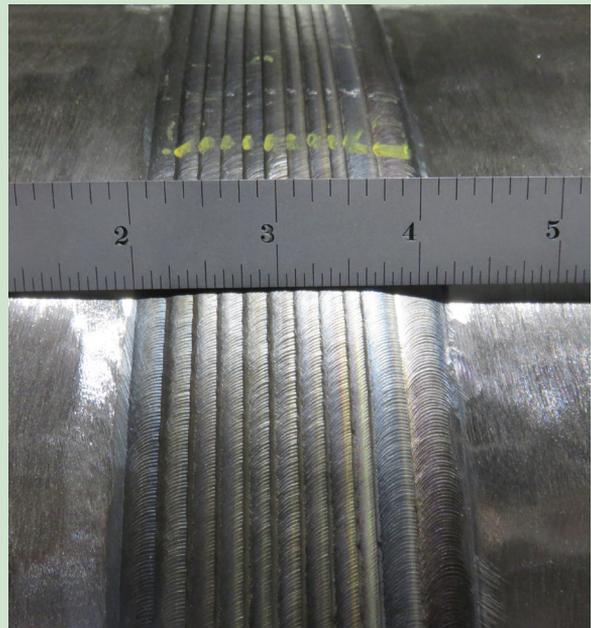
*Fig. 5 — Top — Orbital GTAW narrow groove welding for a nuclear project. Pipe material: P-No. 1. Bottom — Orbital GTAW, 5G cap passes for a seismic oilfield project. Pipe material: P-No. 5A.*
