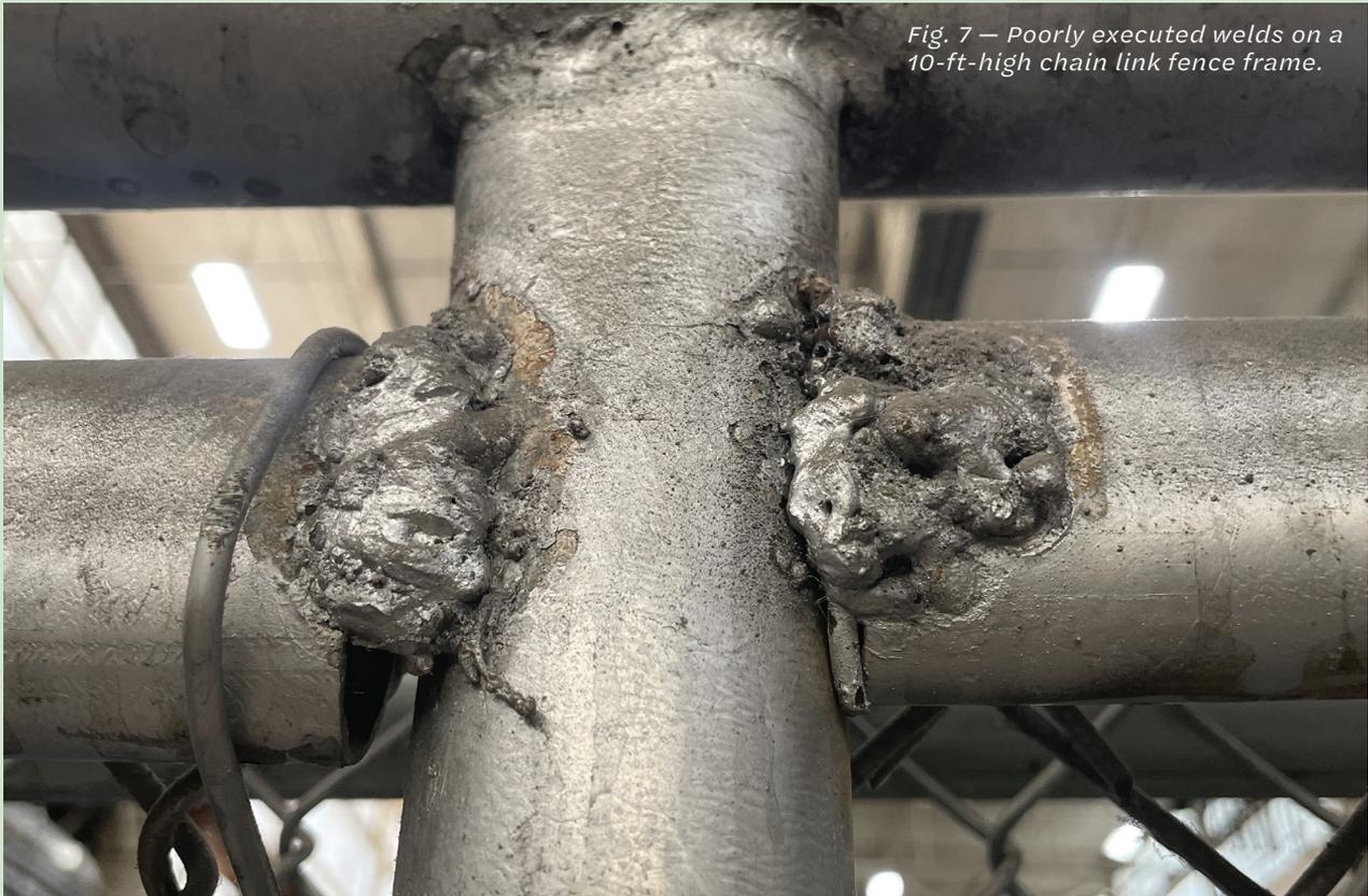
Fig. 7 — Poorly executed welds on a 10-ft-high chain link fence frame.
