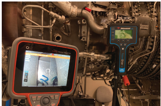
Rhinestahl's FutureDriveNG+ turning tool is now capable of two-way communication with Waygate Technologies' Mentor Visual IQ+ video borescope.
