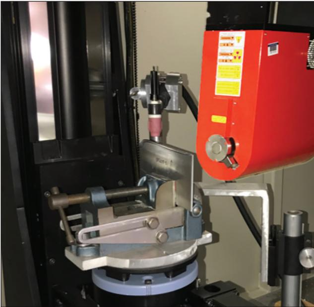
Fig. 2 — Photograph of experimental setup for digital radiography showing an aluminum plate specimen, GTAW torch, and stationary aligned x-ray source (red).
