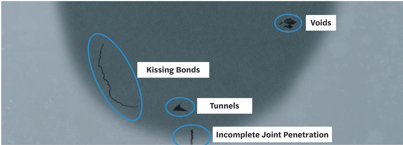
**Fig. 2 – Cross section of a friction stir weld and examples of typical flaws.**
