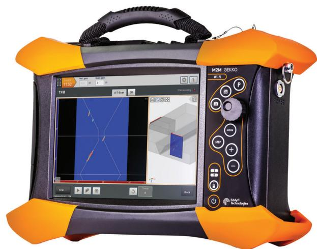
Fig. 2 — The Gekko flaw detector.
