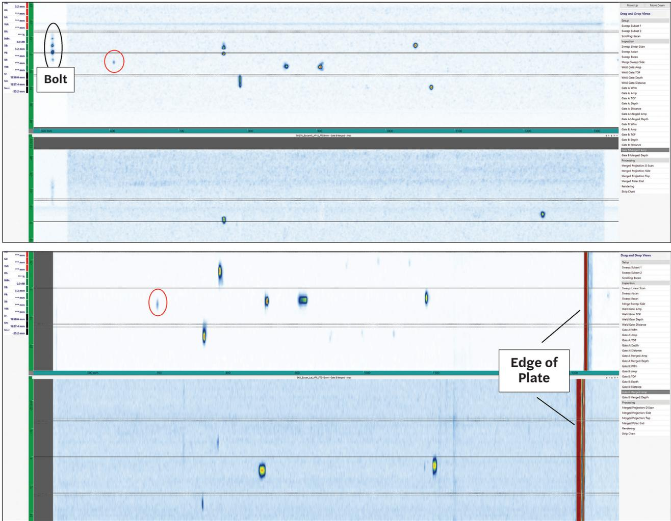
**Fig. 4 — Phased array inspection results on a calibration standard showing six transverse, longitudinal, and oblique notches 0.25 mm [0.009 in.] wide × 2.16 mm [0.085 in.] long, four 45-deg 1.8 mm [0.071 in.] flat-bottom holes, and two small notches (circled in red) 0.25 mm [0.009 in.] wide and 1.27 mm [0.05 in.] long.**
