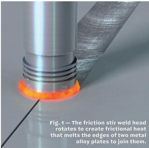
Fig. 1 — The friction stir weld head rotates to create frictional heat that melts the edges of two metal alloy plates to join them.
