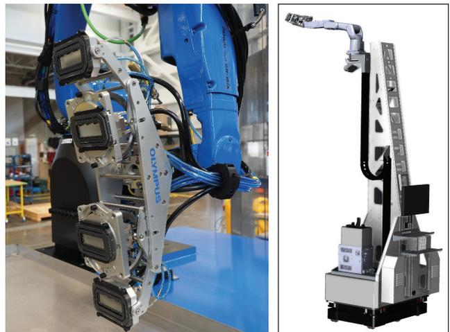
**Fig. 5 (left) — Collaborative robot (cobot) phased array inspection system. Fig. 6 (right) — Phased array automated guided vehicle inspection system.**
