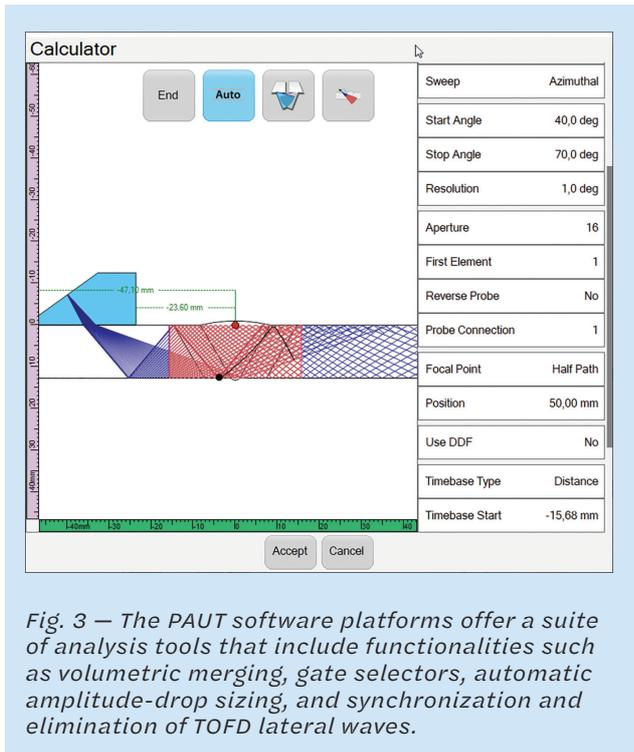
Fig. 3 — The PAUT software platforms offer a suite of analysis tools that include functionalities such as volumetric merging, gate selectors, automatic amplitude-drop sizing, and synchronization and elimination of TOFD lateral waves.
