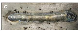
Fig. 13 — Bead appearance according to shielding gas: A — Ar; B — Ar/He mixture; C — He.
