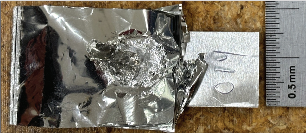
Fig. 11 — MPCC/tab joint produced with 70 lb/in. 2 welder cylinder pressure, 14.71 \mu m amplitude of vibration, and 0.6 s ultrasonic vibration time, showing damaged films around the joint area.
