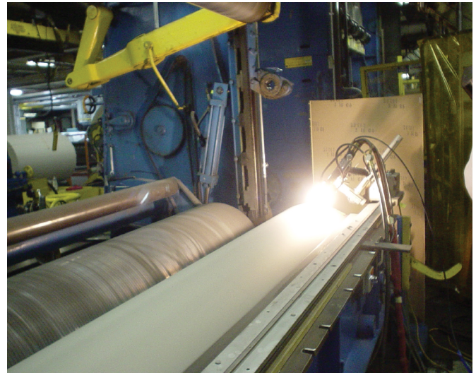
Fig. 3 — Metco 6P on-site flame powder application. (Photo courtesy Hayden Corp.)
