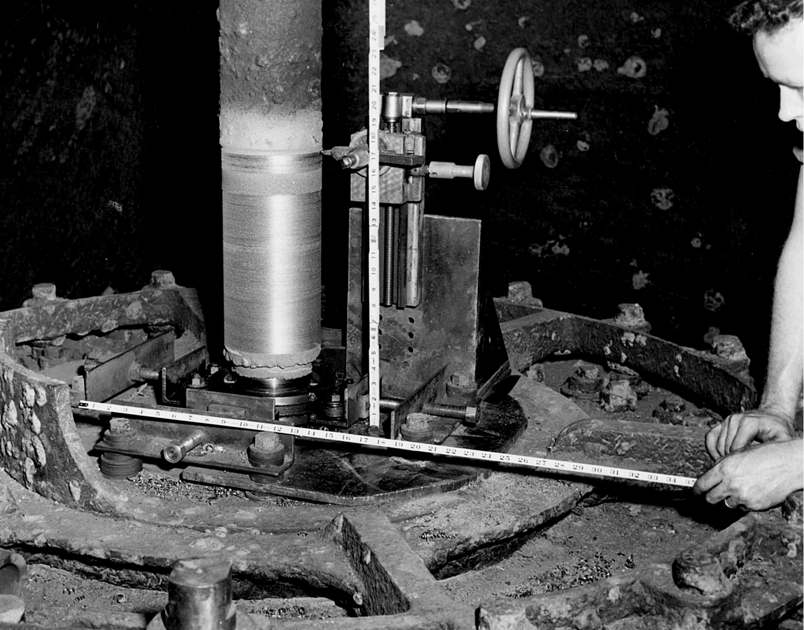
Fig. 4 — Martindale portable lathe for on-site machining. (Photo courtesy of Hayden Corp. archives.)
