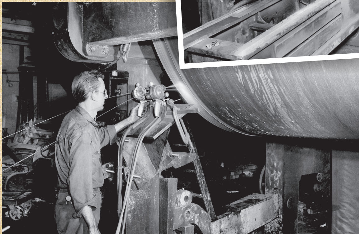
Fig. 1 (top): Metco 12E flame wire application of molybdenum to lathe ways. (Photo courtesy of Hayden Corp. archives.)
