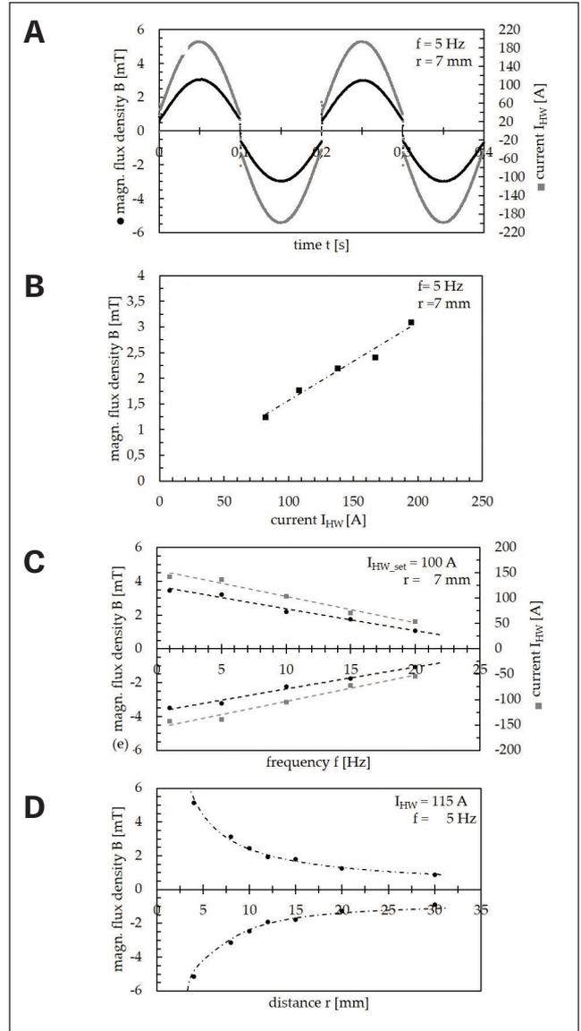
Fig. 3 – Magnetic flux characterization: A – Magnetic flux density  $B$  as a function of the  $I_{HD}$ - $t$ -plot; B – influence of hot wire current  $I_{HW}$  on magnetic flux density  $B$ ; C – influence of frequency  $f$  on hot wire current  $I_{HW}$  and magnetic flux density  $B$ ; D – decreasing magnetic flux density  $B$  as a function of the distance  $r$  to the hot wire.
