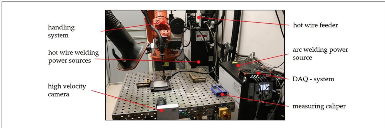
Fig. 1 – Experimental setup.
