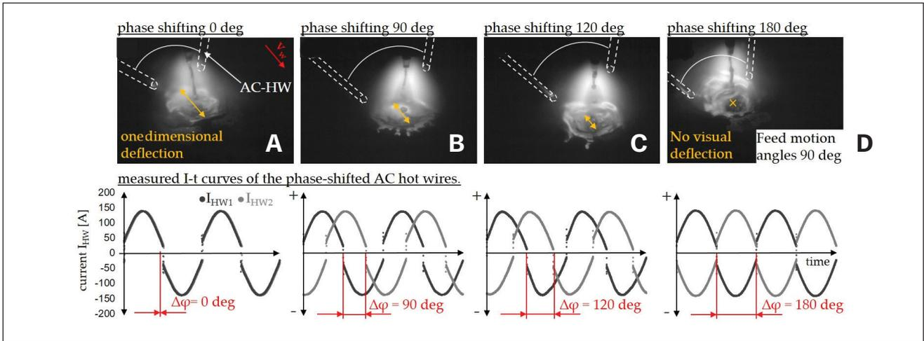
Fig. 5 – Effect of phase-shifted currents  $I_{HW1}$ ,  $I_{HW2}$ , and resulting arc deflection in the GMAW-HW process with two AC hot wires.
