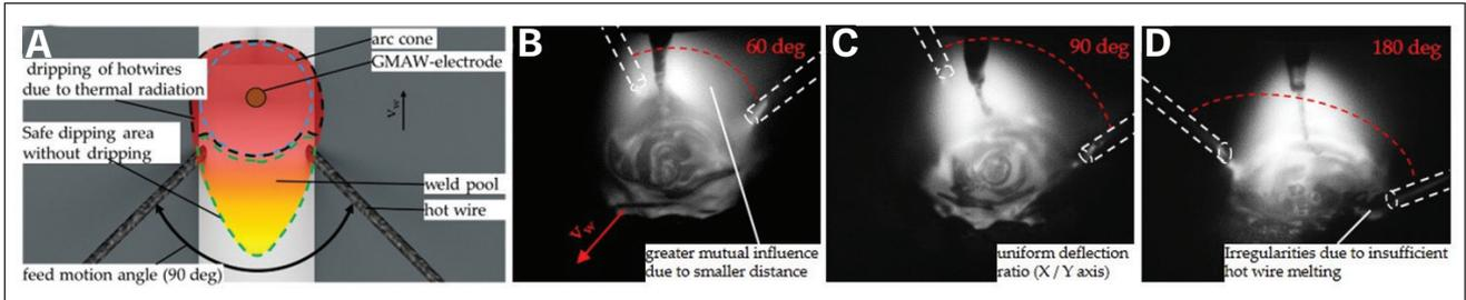
Fig. 4 – Feed motion angles for hot wires: A – Restricted plunging range of hot wires in melting pool; B – high-speed recordings for feed motion angles at 60 deg, C – 90 deg, and D – 180 deg.
