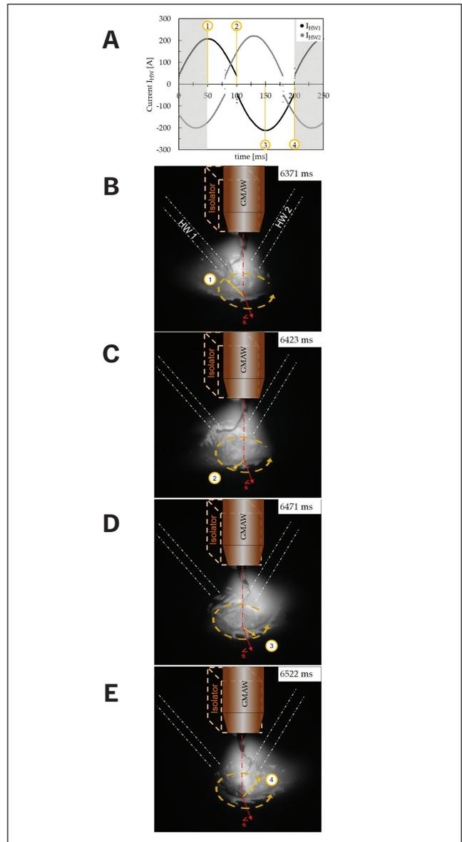
Fig. 6 – A – Two-dimensional arc deflection recordings – I-t plot of the phase-shifted AC hot wires with  $\phi = 120$  deg,  $f = 5$  Hz and characteristic deflection positions 1–4; B – two-dimensional, circular arc rotation in the GMAW-HW process with two phase-shifted hot wires ( $\phi = 120$  deg) using magnetic shielding by a ferritic material (isolator).
