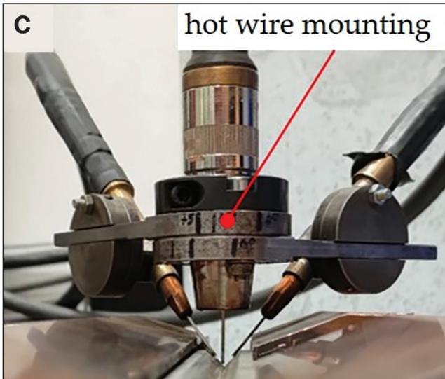
Fig. 2 – Schematic setup: A – GMAW with hot wire mounting; B – fixed parameters for hot wire positioning; C – experimental setup with hot wire mounting.
