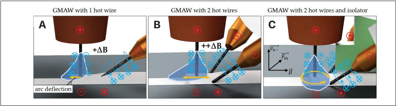
Fig. 8 – Schematic magnetic field lines during the GMAW-HW-process: A – One hot wire; B – two hot wires; C – two hot wires with isolator.
