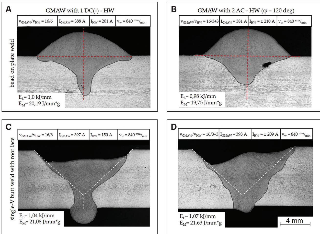
Fig. 7 – Comparison between the GMAW-HW process with one DC hot wire and GMAW-HW process with two phase-shifted AC hot wires ( $\varphi = 120$  deg) for constant line energy  $E_L$  based on the example of bead-on-plate welds (A, B) and single-V butt joints with root face (C, D).
