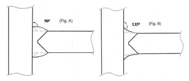
**Response**: The intent of a reinforcing fillet weld is to provide a gradual transition of the weld face to the base metal. Figure A does not accomplish this purpose. Figure B meets this intent.
