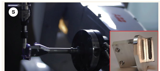
Fig. 5 — Robotic application of UV-curing resin together with finish-sprayed test component.
