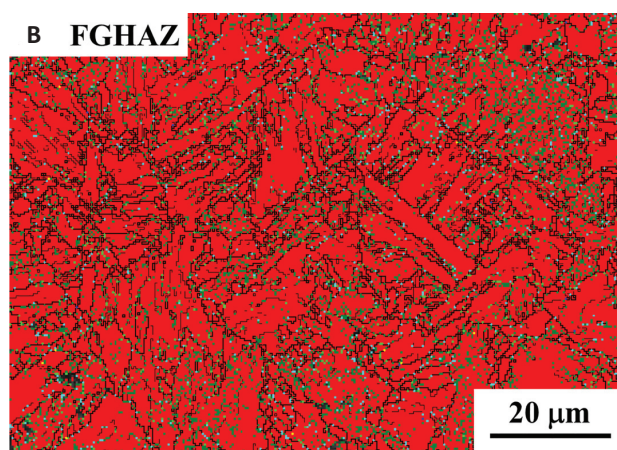
Fig. 11 — The EBSD phase distribution maps: A — CGHAZ; B — FGHAZ; C — ICHAZ.
