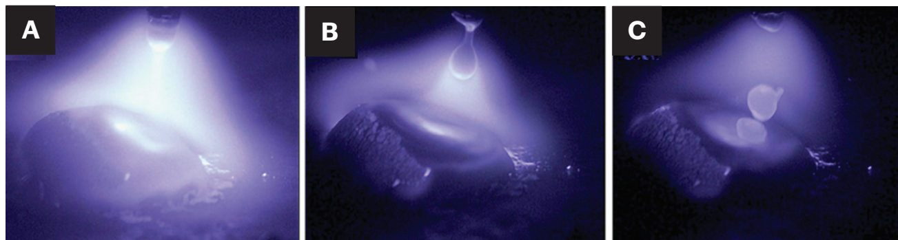
Fig. 12 — Natural radiation lighting with an 850 nm LWP filter of pulsed GMAW of 4043 aluminum in pure Ar: A — Peak current; B — downslope after peak; C — droplet formation during background current.
