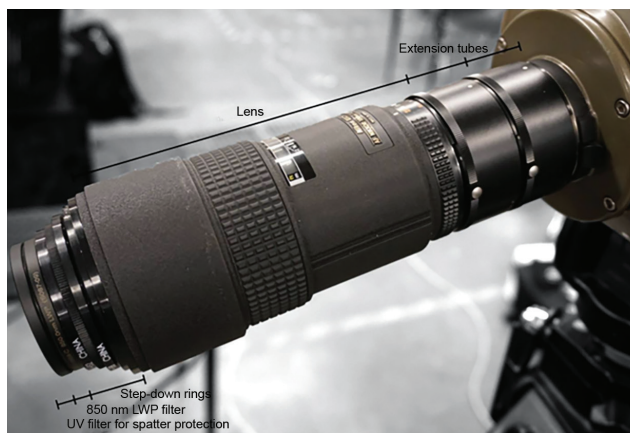
Fig. 5 — Example configuration of 180-mm focal length lens (F-mount) with two 25-mm extension tubes, step-down rings, \Phi 52-mm, 850-nm LWP filter, and \Phi 52-mm UV filter for spatter protection. Some applications might benefit from a circular polarizer between the LWP and the UV filters.
