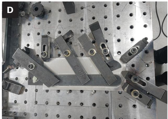
*Fig. 3 – A – Laser welding setup; B – weld of interface rim; C – clamping strategy of center weld; D – representative clamping strategy of periphery welds.*
