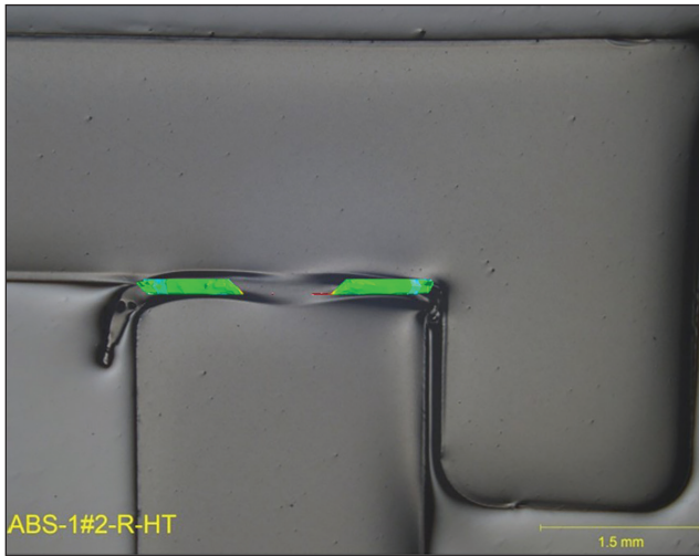
Fig. 22 — Cross section of welded ABS part with model flow overlaid.
