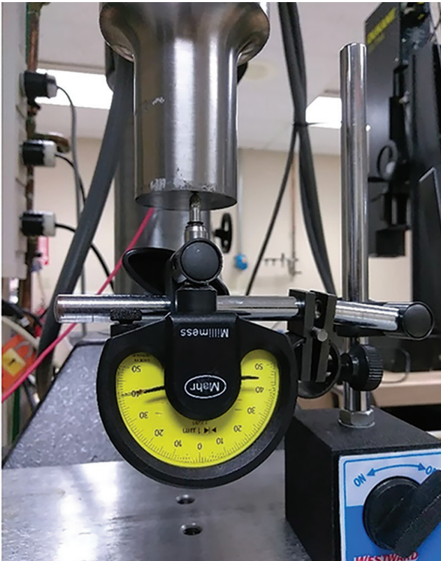
Fig. 3 – Method for measuring amplitude at the ultrasonic sonotrode face using a displacement gauge.
