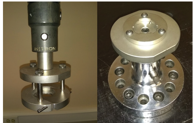
Fig. 16 – Tensile testing tooling: top (left); bottom (right).
