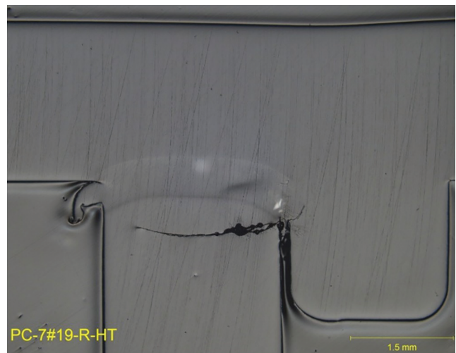
Fig. 17 – PC, 20 kHz, 0.44-mm collapse, 374-N trigger force, 0.035-mm amplitude.
