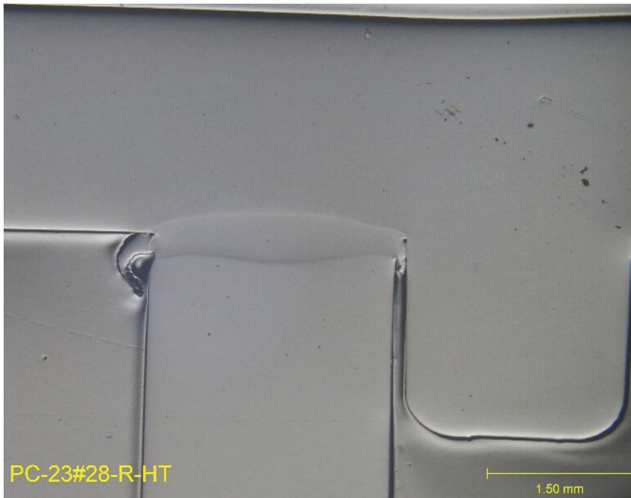
Fig. 20 — PC weld with intermolecular diffusion.
