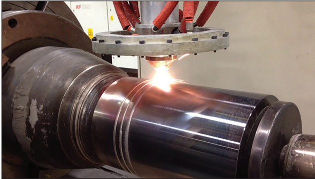
Fig. 1 – Laser Cladding Experiment (Ref. 21).
