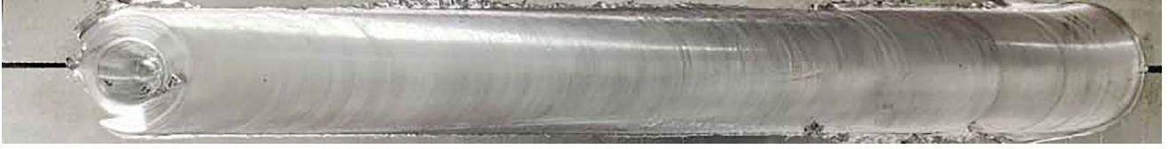
Fig. 2 – Friction stir welding weld morphology of 2219-T8 aluminum alloy.
