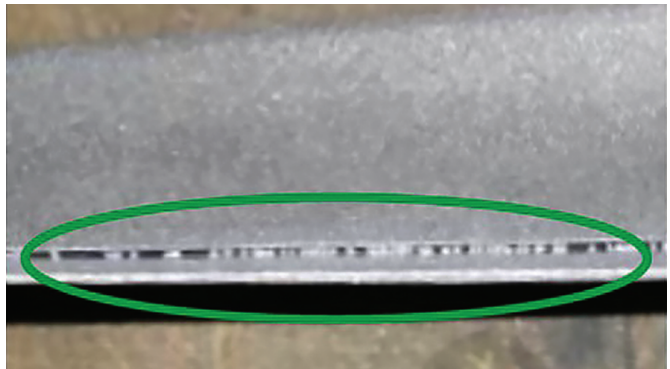
Fig. 7 – 20 mesh alumina grit trapped in a turbine blade trailing edge cooling slot.
