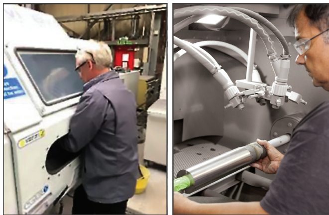
Fig. 3 – Manual and semiautomated grit-blasting processes.
